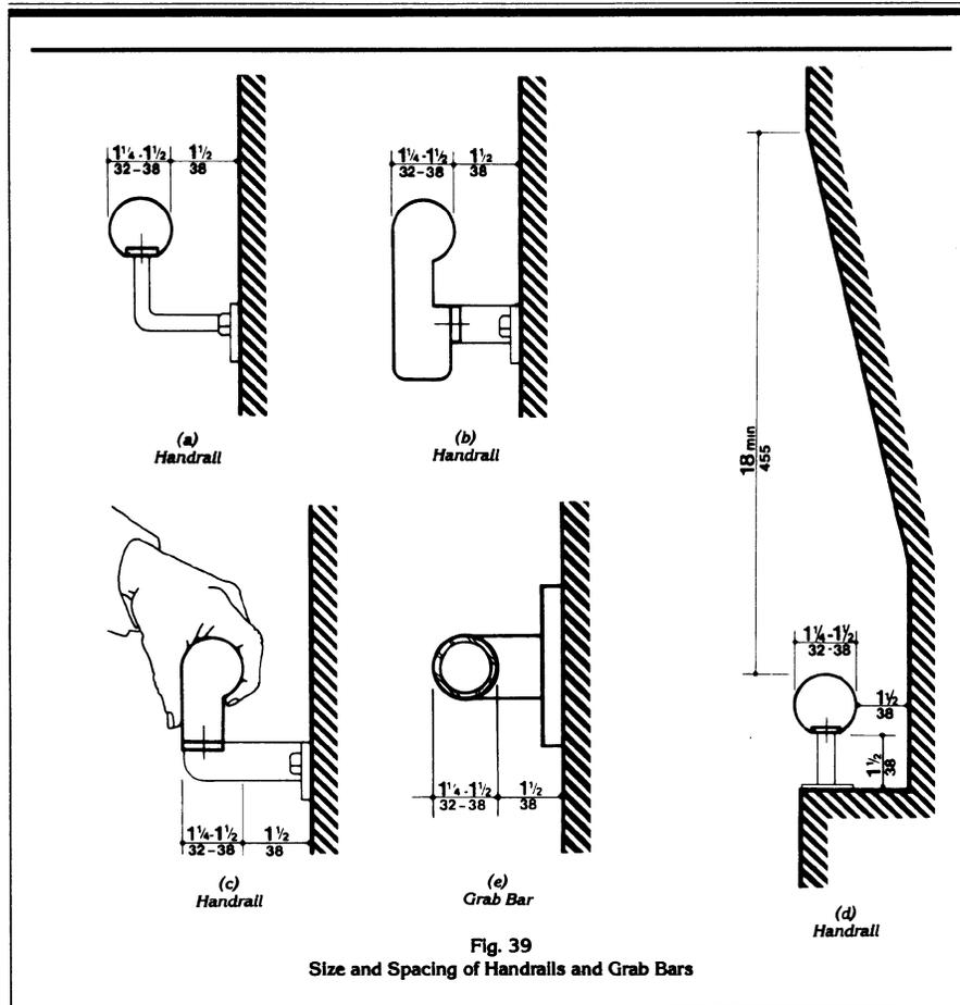
**4.26.4 Eliminating Hazards.** A handrail or grab bar and any wall or other surface adjacent to it shall be free of any sharp or abrasive elements. Edges shall have a minimum radius of 1/8 in (3.2 mm).
