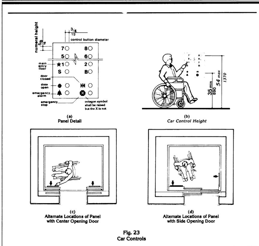
(4) Location. Controls shall be located on a front wall if cars have center opening doors, and at the side wall or at the front wall next to the door if cars have side opening doors (see Fig. 23(c) and (d)).
